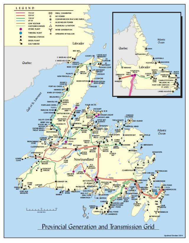
Figure 1 - Hydro's Generation and Transmission Infrastructure
