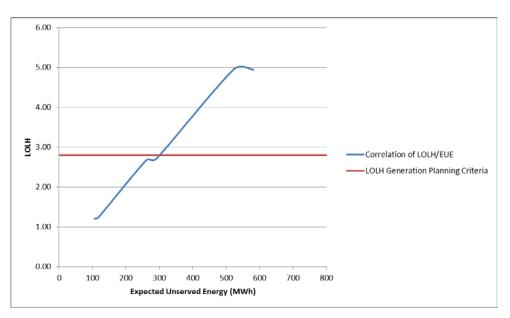
Figure 2 – Illustration of EUE vs LOLH
